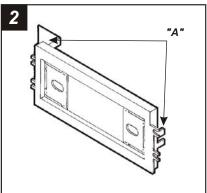
Cut and remove all mounting tabs on the Radio Housing EXCEPT tabs "A". The mounting tabs can be identified by the stamped letter on the back of each tab. Skip to the Installation Instructions for ALL VEHICLES on Page #5.
